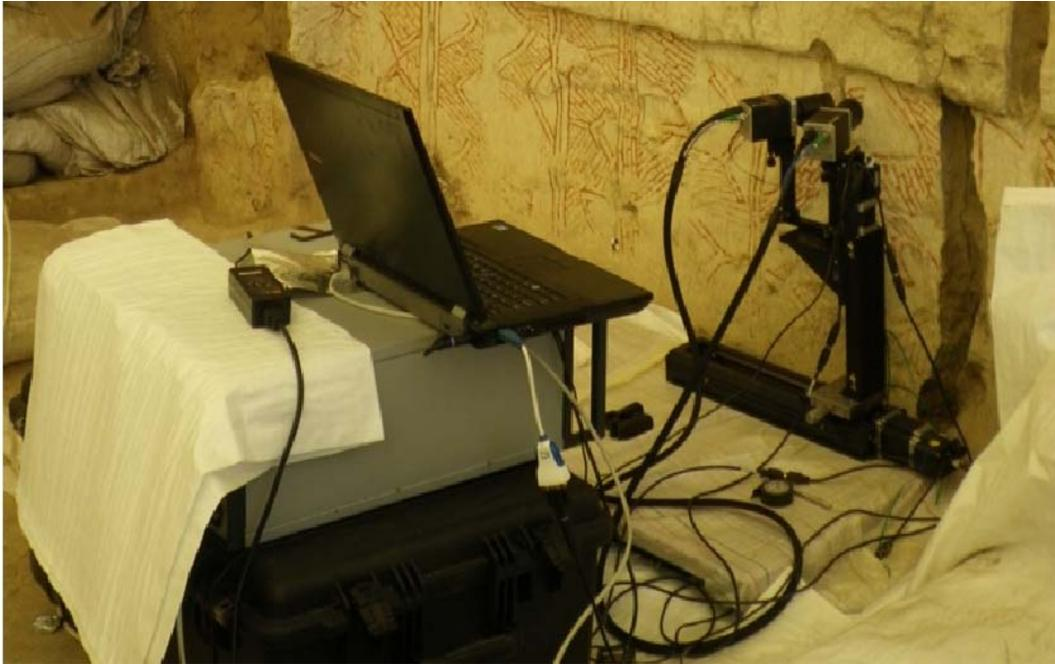
Figure 173. Photograph of a picometrix T4000 pulsed imaging system scanning a wall painting in Çatalhöyük, South Area, Room 80.
