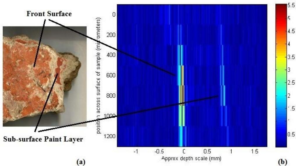
Figure 172. (a) Photograph of multi-layer mud plaster specimen from Area 4040 Space 1006, East wall F 3008, Unit (16080) and (b) a line scan of deconvolved data representing the internal structure of the wall plaster.
